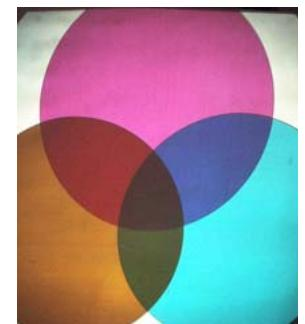
*Fig. II-20 - Overlapping arrangement of yellow, cyan and magenta color filters on an overhead projector. In the overlapping regions, color subtraction results in green, red and blue light.*
