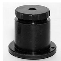
Fig. III.31. Detector Calibration Standard
